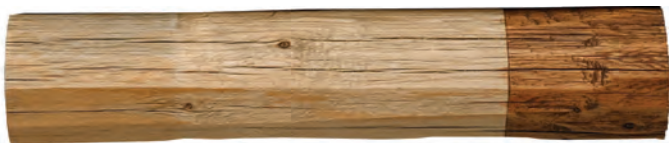
Prep Method used was Power Washing followed by a 3M® non-woven pad.
