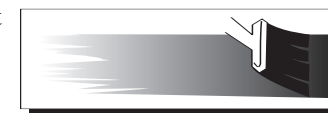
Feathering Technique, use only if stopping in the middle of a log is unavoidable.
